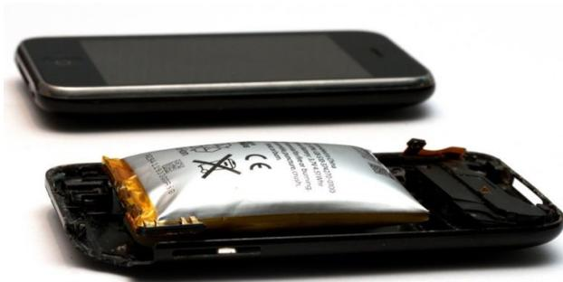
Expanded lithium-ion polymer battery (wikimedia.org)
